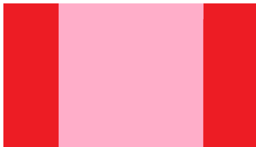
Illustration of a square ROI scaled and embedded in a standard 16:9 video.
